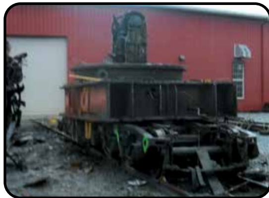
Only the cable drum, crane pivot plate and crane main base plates remain. January 19, 2023
